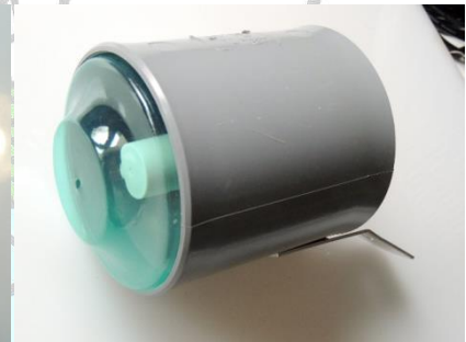
Figure 7: Radôme de protection
